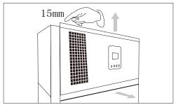
3. Remove all inner and exterior screws to release the top decoration plate.
