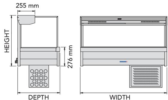
Note: For SRX model range overall height dimensions, add height of motor cage (450 mm).
