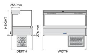
Note: For SRX model range overall height dimensions, add height of motor cage ( $450\ \text{mm}$ ).
