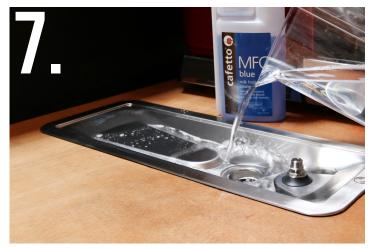
Pour the remaining diluted solution into the rinser slowly and allow the solution to drain. This will clean the drain piece and drain hose.
