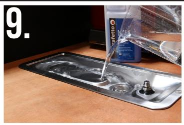
Once complete and all milk residue has been removed, give the entire unit a final rinse with clean water.
