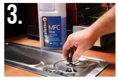
Unscrew the spray valve from the rinser body.
