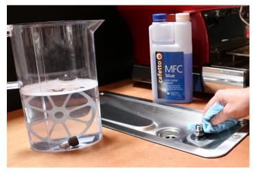
Dip a soft cloth into the diluted cleaning solution and use to wipe down the surfaces of the rinser. Remove soaking parts from cleaning solution and rinse.
