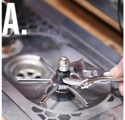
(A) Using an adjustable wrench, locate the 2 notches at the base of the spiniet
