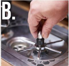
(B) Replace the Spinjet by attaching (C) Tighten with adjustable wrench to the spray valve.
