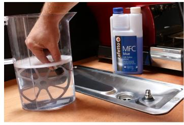
Add the removed parts to the Daily Milk Frother Cleaner solution. Allow the parts to soak while cleaning the remainder of the rinser.
