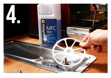
Remove the Actuator Plate.
