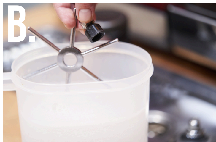
(B) After 10 minutes, remove the Spinjet tip and actuator star from cleaning solution and rinse thoroughly with clean water.
