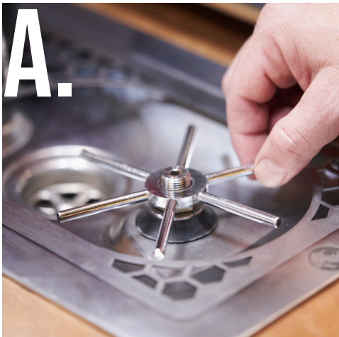
(A) Replace the actuator star over the valve body.
