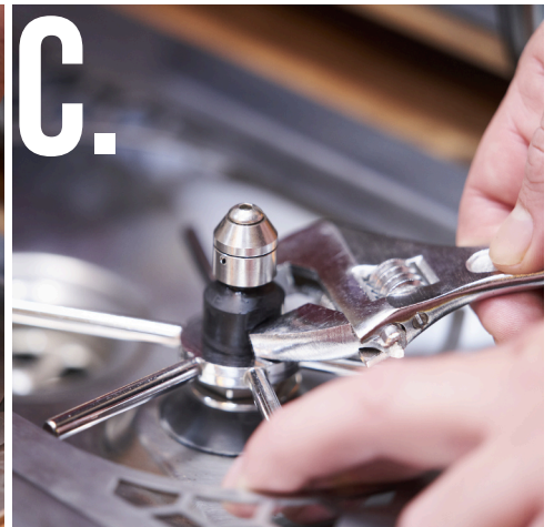
(C) Tighten with adjustable wrench & Replace the drain tray.
