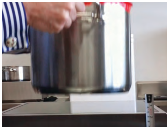
Heavy drop test on tough NEG glass*
