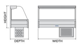
Note: For CRX model range overall height dimensions, add height of motor cage (450 mm).
