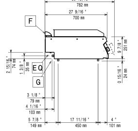
EQ = Equipotential screwG = Gas connection
