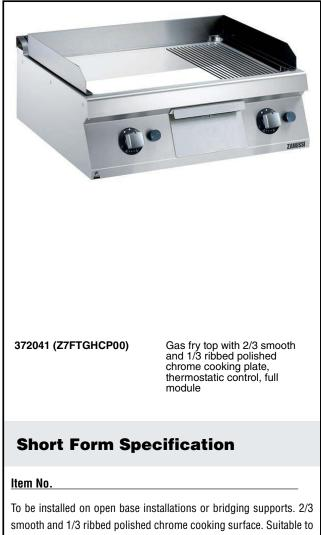
smooth and 1/3 ribbed polished chrome cooking surface. Suitable to be used with Natural or LPG gas. Temperature range from 100°C to 280°C. Removable drawer below the cooking surface for the collection of grease and fat. Exterior panels in stainless steel with Scotch Brite finish. One piece pressed work top in 1.5 mm thick stainless steel. Right-angled side edges to allow flush-fitting junction between units.
